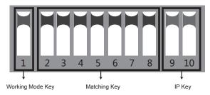
**Button 1** changes the mode of the device. UP is access point (AP) mode for use with your recorder, PC, etc.. DOWN is for use with your camera.
