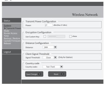
**Transmit Power Configuration:** The default is the maximum value, the transmit power should be reduced appropriately when the signal is too strong.
