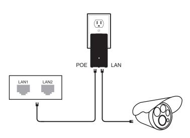
The bottom of the adapter has two RJ45 connections. One marked POE and one marked LAN.
