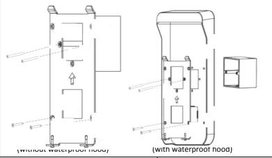
6. Fasten the access control terminal to the bracket hook.
