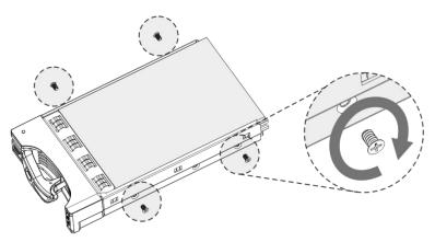
Step 4 Put the drive tray back in the DVR and lock the handle. Figure 2-19
