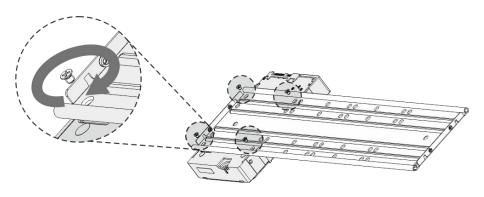
Step 5 Fix other disks on the bracket as needed.
