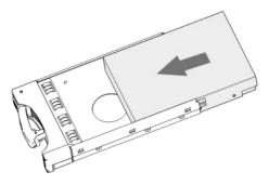
Step 3 Fix the disk in the drive tray with the four screws.
