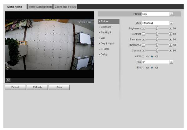
Figure 4-33 Camera conditions (PTZ camera)
