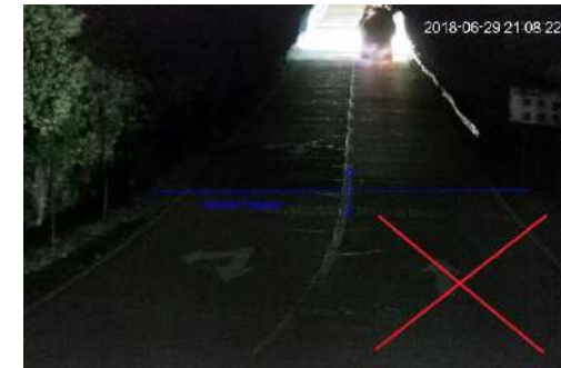
In the dark, the detecting rate of color mode is low. You need to switch it to black-and-white mode
