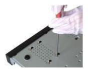
(5) Turn the device upside down; fix the screws to secure the HDD on the bottom of the chassis.
