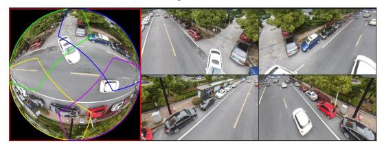
In Figure 4-77, you can adjust the color pane on the left pane or use your mouse to change the position of the small images on the right pane to realize fish eye de-warp.
