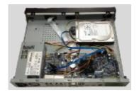
(4)Connect the HDD cable and power cable.
