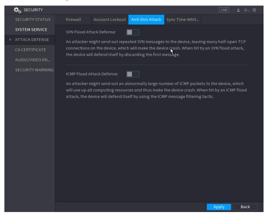
Figure 4-247 Anti-Dos attack interface
