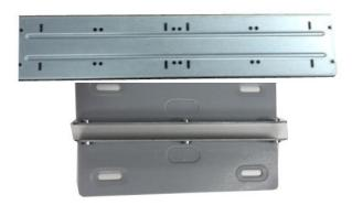
(2) Take off the bottom of the HDD bracket and CD-ROM bracket.
