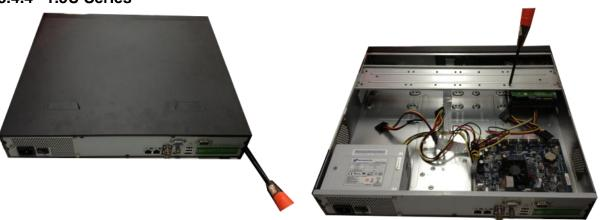
(1) Use the screwdriver to loose the screws of the rear (2) Put the HDD to the HDD bracket in the chassis
