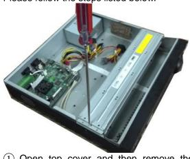
(1) Open top cover and then remove the HDD bracket
