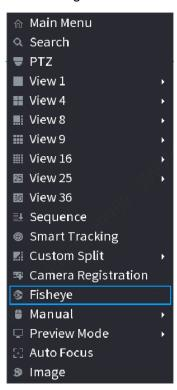
Now you can see an interface shown as Figure 4-76. You can set fish eye installation mode and display mode. There are three installation modes: ceiling mount/wall mount/ground mount.
