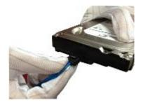
③ Connect the other end of the HDD data cable and the power cable to the HDD.
