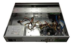
3 Connect to the HDD data cable to the main board and the HDD port respectively. Loosen the power cable of the chassis and connect another end of the power cable to the HDD port. and then line up the four screws to the four holes in the HDD. Use the screwdriver to fix the screws firmly to secure HDD on the HDD bracket
