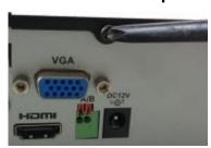
①. Loosen the screws of the upper cover and side panel.
