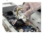
② Connect the one end of the HDD data cable and the power cable to the mainboard.
