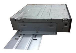
(5) Install SATA burner. Line up the SATA burner to the hole positions.
