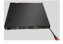
5) Put the cover in accordance with the clip and then fix the screws on the rear panel and side panel.
