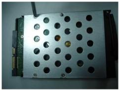
①Use 4 screws to secure the HDD
