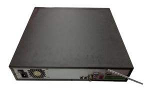
Use the screwdriver to loose the screws of the rear panel and then remove the front cover.
