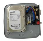
② Place the HDD in accordance with the four holes in the bottom.
