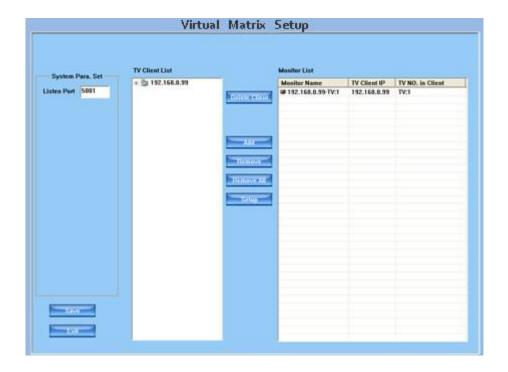
The IP "192.168.0.99" here is one of the PC you installed TV client on. After you filled the CMS IP "192.168.0.192" (the sever end, mentioned before) in login interface when running TV client, its IP will be displayed here automatically.
