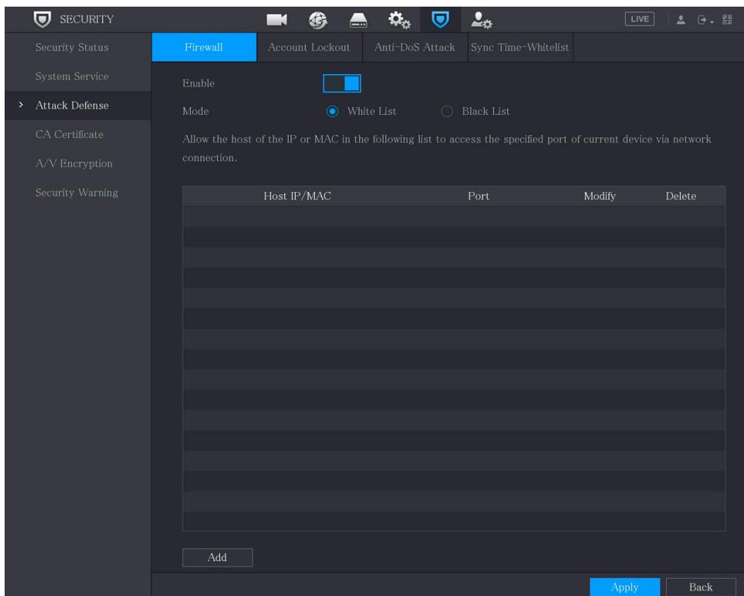
**Step 2** Select **Enable** to enable firewall.
