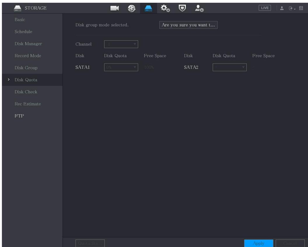
**Step 2** Select the channels you want to configure, and select quota from the drop-down list of corresponding HDD.
