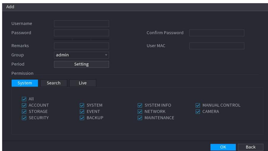
**Step 3** Configure the settings for the parameters of adding a user account.
