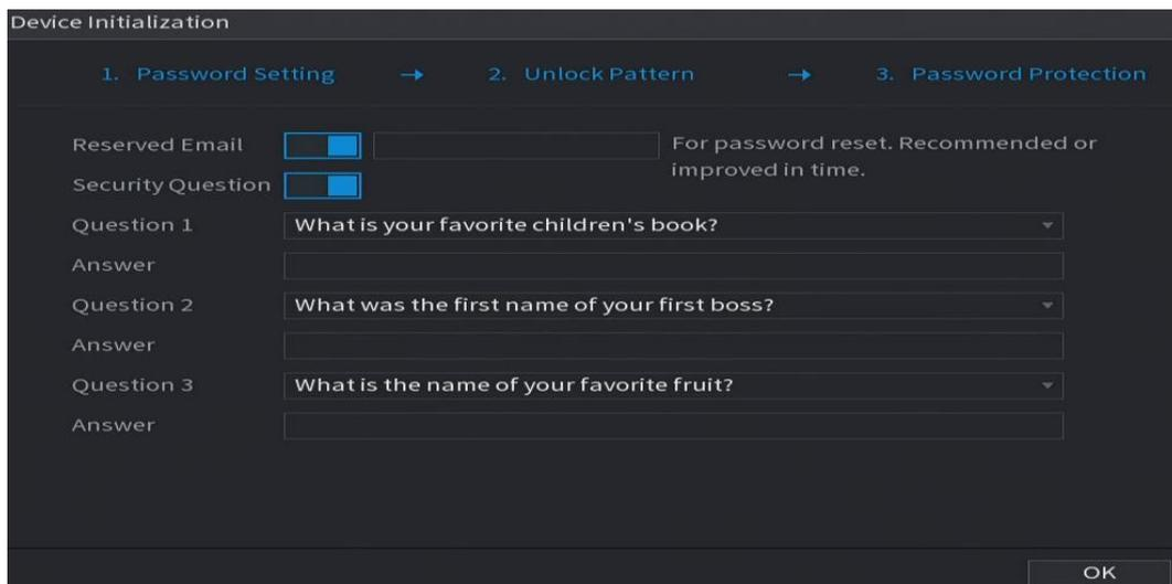
Step 12 Configure the protection parameters for password.
