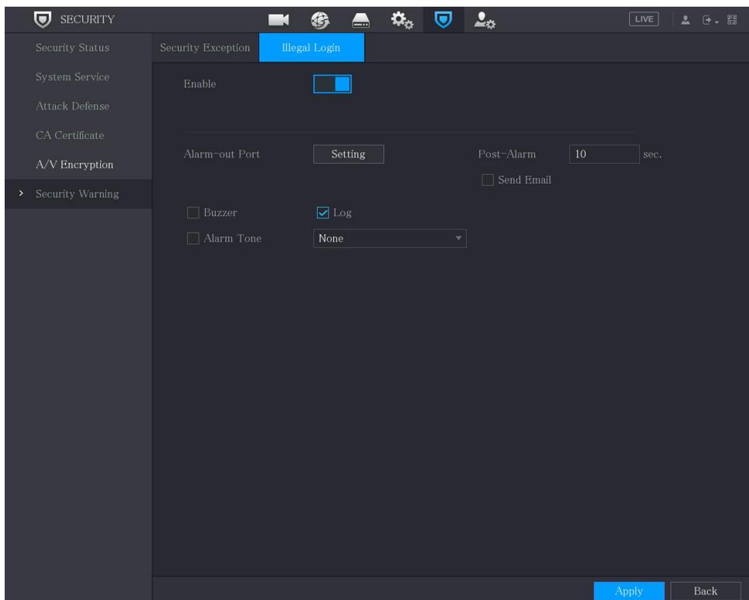
**Step 2** Select **Enable** and configure parameters.
